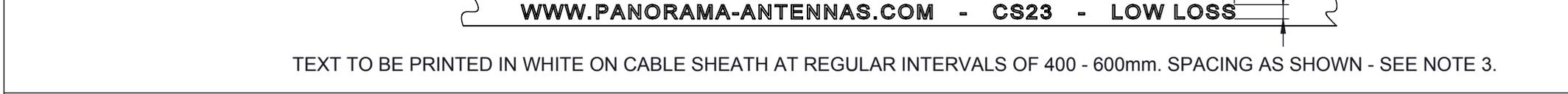
TEXT TO BE PRINTED IN WHITE ON CABLE SHEATH AT REGULAR INTERVALS OF 400 - 600mm. SPACING AS SHOWN - SEE NOTE 3.
