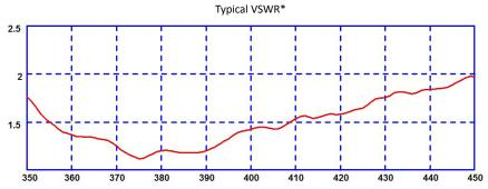
VSWR shown on a 1x1m (3'x3') ground plane with 5m of CS23 (RG58 c/u) cable
