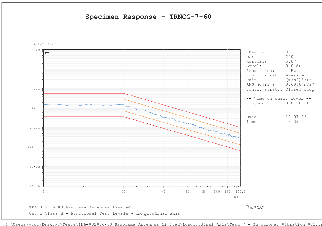
Test 7 - Functional Vibration Test Longitudinal Axis Vibration and Shock Tests
