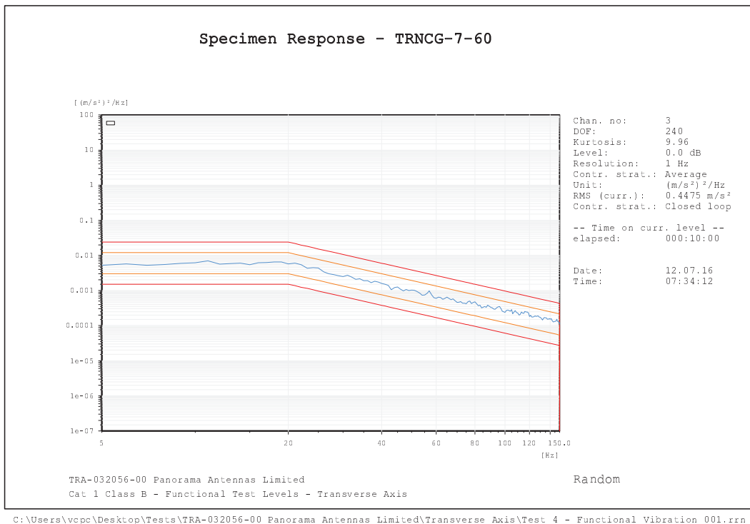
Test 4 - Functional Vibration Test Transverse Axis Vibration and Shock Tests
