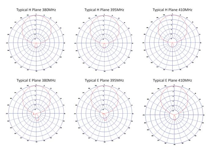
\*Patterns measured in free space with 1m of CS23 cable
